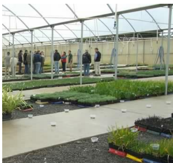
Top: Boom spray calibration at Narromine Transplants, Bottom: catch cans deployed for testing at Larkman Nurseries
